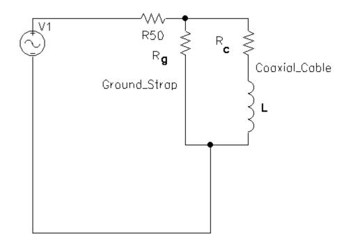
$I_{\text{ground strap}} = I_{\text{resistor}} * (R_c + j\omega L) / (R_c + j\omega L + R_g)$  (Current Divider)
